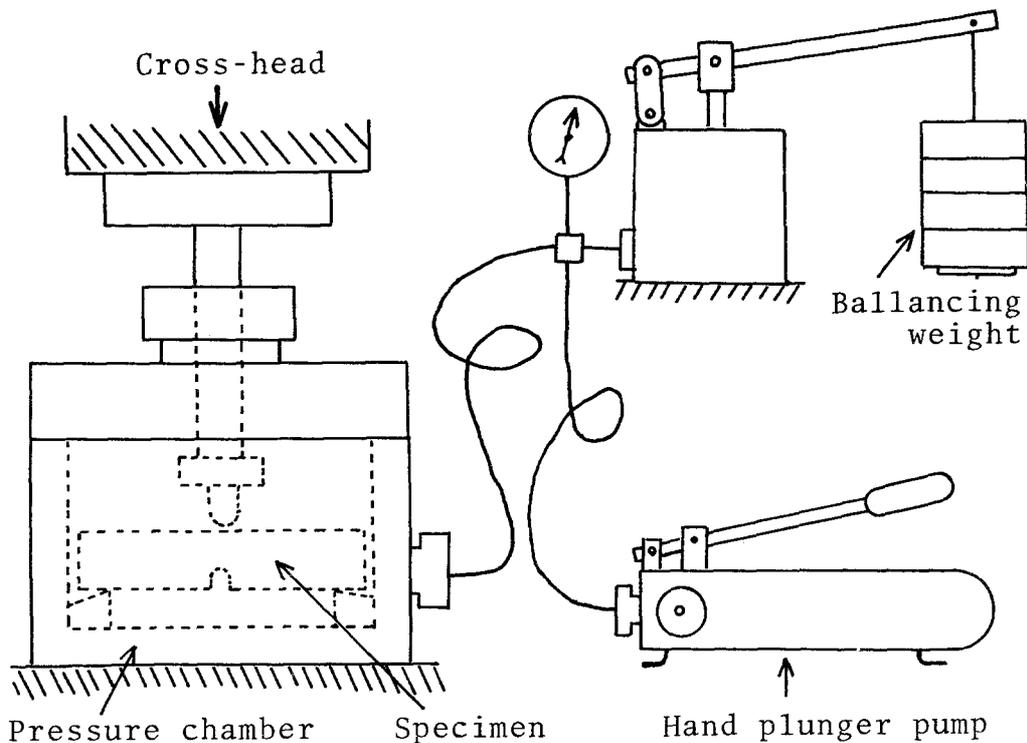
Figure 2 Schematic diagram of the apparatus used in the three-point bending test under hydrostatic pressure.
