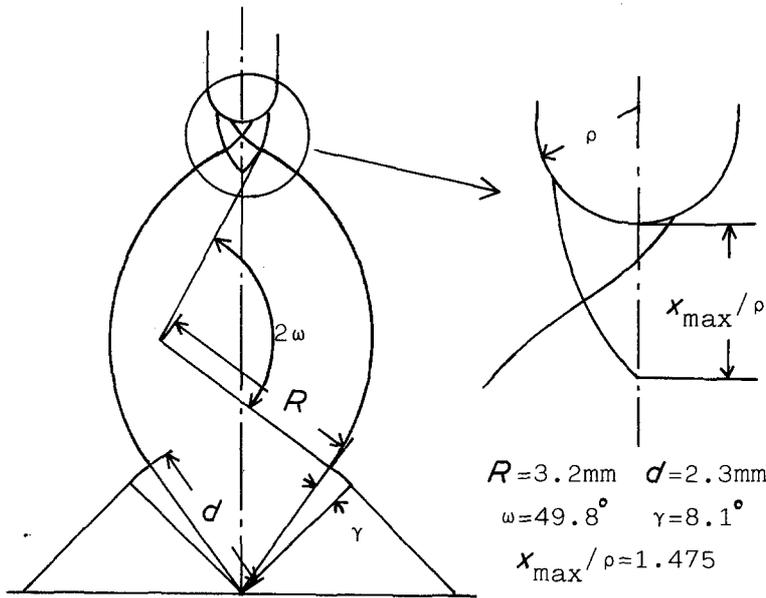
Figure 12 Slip-line field at general yield for a round-notched bar subjected to three-point bending.
