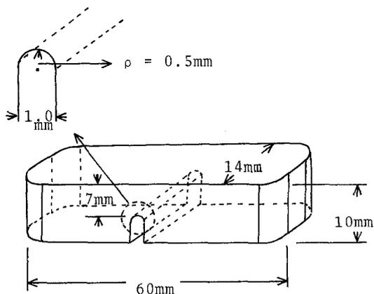
Figure 1 Shape and dimensions of test samples.
