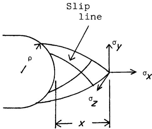
Figure 10 Definition of stress components.
